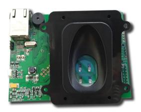
FS84C has 1 output channel (for external relay control) and 2 input channels (for door sensor and switch). So it can be used as a fingerprint access control device.
